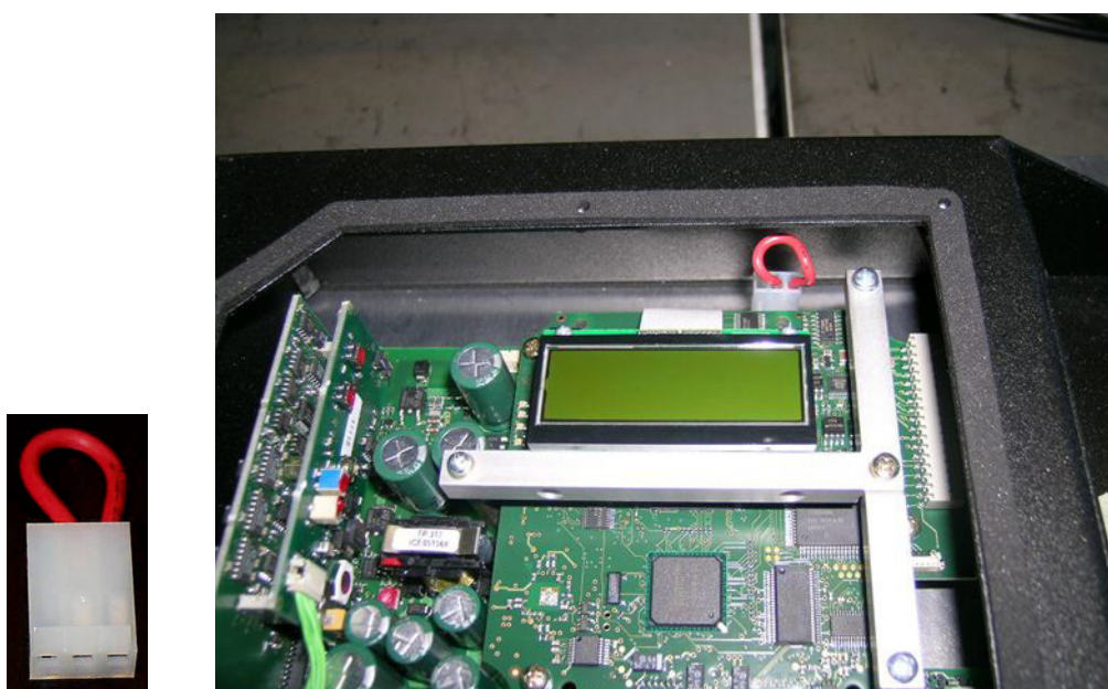
Figure 68 - Connecting the power supply jumper for external Vdc operation
