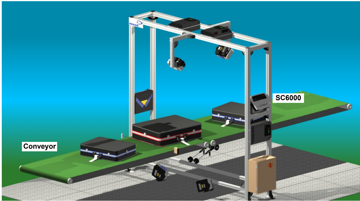
Figure 41 - Large Synchronized Network Reading Station
